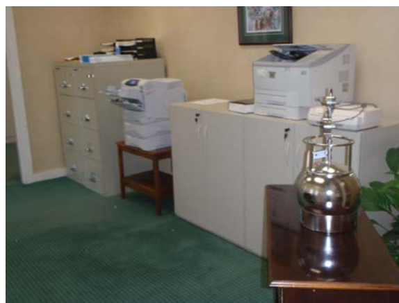
Figure 3. SUMA Canister used for collecting 24-hr composite indoor air sample
