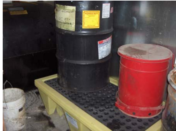
Figure 2. Drum Storage with Secondary Containment
